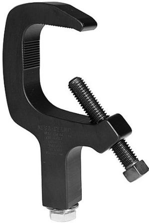
The Mega-Clamp is the world's new standard theatrical lighting C-Clamp. The Mega-Clamp is created from high tensile, aircraft grade, extruded aluminum; so it's both stronger and lighter than cast iron damp. The Mega-Clamp's safety factor far exceeds industry standards, breaking at over 2-1/2 tons at an independent testing laboratory. It is half the weight and twice as strong as most cast iron damp.
